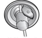
Inlet Valve with escutcheon being tightened into place with installation wrench
